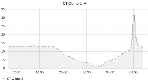
Example of current consumption for single phase.
