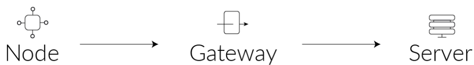
Figure 17 IoT system components.
