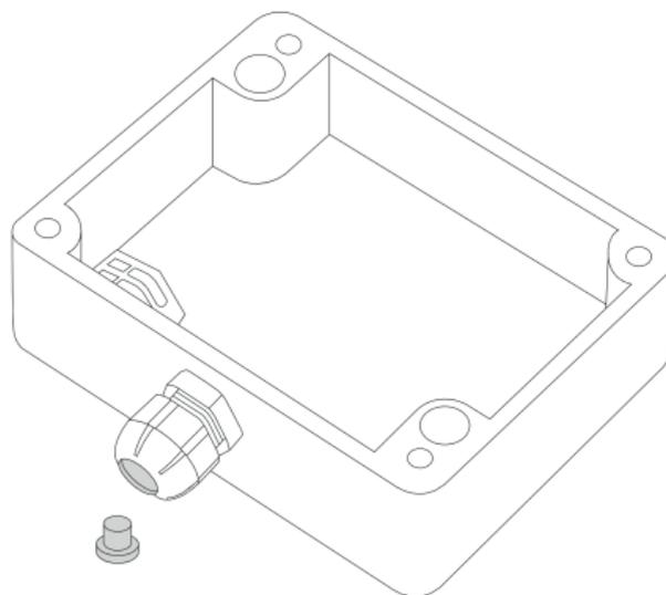
Figure 10 Device with removed top cover and PG7 cap marked.
