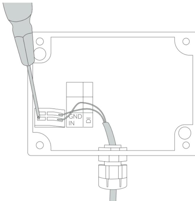
Figure 12 Connecting input cable instructions.
