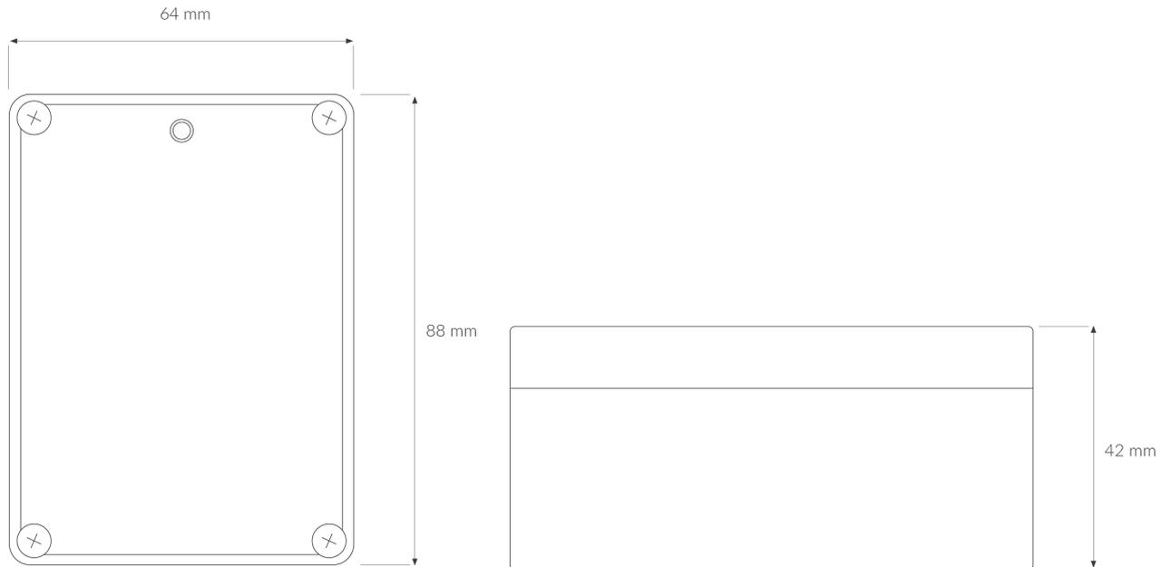
Figure 4 Dimensions of the device.
